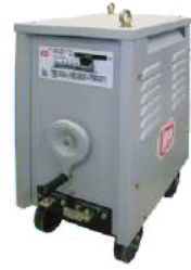
AC 200A HEAVY DUTY - MOVING CORE Input: Single / Two Phase Electrode: Upto 3.15mm Duty Cycle: 40% Two Years Warranty for Transformer
