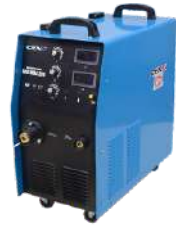
MIG/MAG 200 PROFESSIONAL MACHINE IGBT Inverter Technology; DC Output Input: Single Phase; Wt. 27.0Kgs. Built in Closed Wire Feeder Duty Cycle: 60% Suitable for Aluminium Welding
