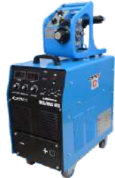
MIG/MAG 500 / 630N (HD) PRODUCTION MACHINE IGBT Inverter Technology; DC Output Input: Three Phase; Wire Dia: upto 3.0mm External 4 Roller Wire Feeder Duty Cycle: 60%; MMA Possible Electrode Usable: Upto MS 6013-5.0mm Suitable for Aluminium Welding
