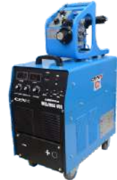
MIG/MAG 400 PRODUCTION MACHINE IGBT Inverter Technology; DC Output Input: Three Phase; Wt. 30.0Kgs. External 4 Roller Wire Feeder Duty Cycle: 60%; MMA Possible Electrode Usable: Upto MS 6013-4.0mm Suitable for Aluminium Welding
