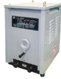
AC 300A / AC 400A HEAVY DUTY - MOVING CORE Input: Two Phase Electrode: Upto 5.0mm Duty Cycle: 40% Two Years Warranty for Transformer
